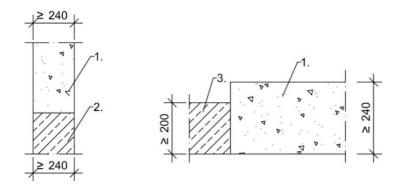
Cables  $\emptyset \le 80$  mm, cables bundles  $\emptyset \le 100$  mm with cables  $\emptyset \le 21$  mm and cable trays with intumescent wrap (wrap width = 500 mm)
