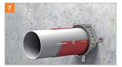
Mount each mounting point with the appropriate dowels to the wall / underneath the floor. For lightweight partition walls, work with mineral fibre seal and threaded rods M6 or M8. Finally, apply an identification sign to the seal.
