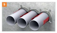
Special application: Multiple installation of up to 3 pipes lined up next to each other (PVC, PE and PP) with an outer pipe diameter of  $\leq$  75 mm. The distance between the individual pipes must be max. 15 mm.
