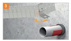
Bend the metal wrap with a fastening hook by counting the necessary metal link according the table. Mount the fastening hook to the upper side of the metal wrap. Make sure the fastening hook is flush with the metal wrap on the left side. Break off the metal wrap by moving it back and forth. By doing so, no additional tools are necessary.
