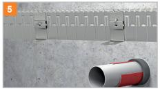
Mount the fastening hooks to the appropriate positions. Insert the  $90^\circ$  bended lug through the opening and bend it back so that the hook is fixed tightly.
